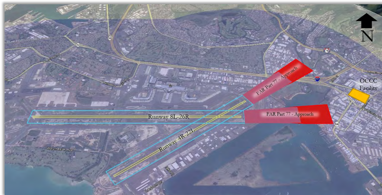
Exhibit 4: Part 77 Surfaces HNL Runways 8L-26R and 4R-22L—Isometric View
