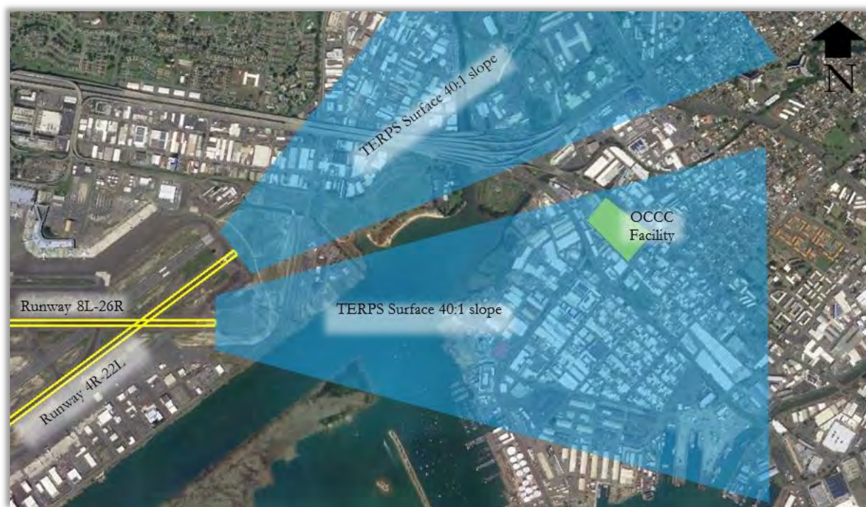
Exhibit 4: TERPS Surfaces—HNL Runways 8L-26R and 4R-22L—Plan View
