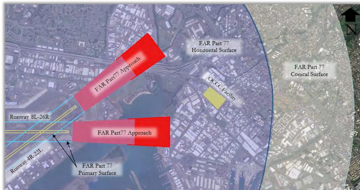
Exhibit 3: Part 77 Surfaces at HNL—Plan View
